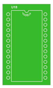
As seen in the drawing on the Left the EPROM has a small notch in the Top. You will also find a similar notch in the white silkscreen on the PCB (the drawing on the Right) at the U18 location. This indicates the correct orientation for the EPROM.
