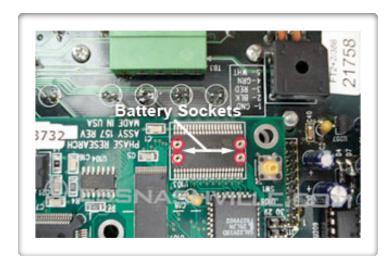
And here you can see the 4 battery sockets, where the leads of the battery go.
