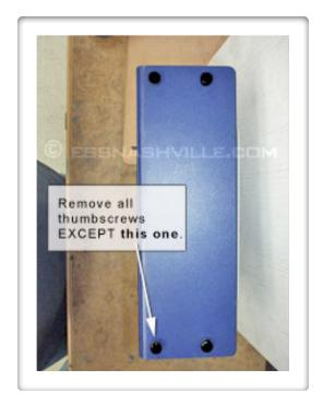
If your timer has only 2 thumbscrews on each side as shown in this photo, remove or loosen the top one. Leave the bottom one, closest to you, attached but loosened slightly.
