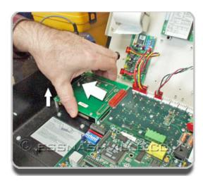
While pulling the Printer board away from the Main board, lift the back side to clear the components on the bottom.
