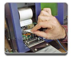
Start the tip of the paper into the slot on the inside of the printer door.
