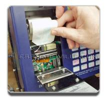
When you see the tip of the paper at the bottom of the printer, gently pull it until 4 to 5 inches is hanging out.
