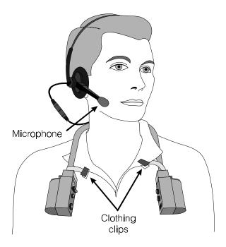
Figure 4. Correct wearing of the COM400CC
