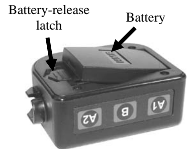
Figure 6. Belt-pac battery-release latch
