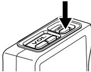
2. While holding R and T1 simultaneously, press the power button to turn on the Order Taker. The Order Taker enters manager setting mode where the indicators and buttons have different functions than in normal operation. You can hear "Connecting center module A" and power indicator is an alternate blinking of red and green. Also the Lane indicator A is blinking yellow.
