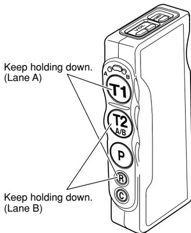
When you want to register the manager in another center module in a double-drive-thru environment, while holding R and T2 simultaneously, press the power button to turn on the Order Taker. You can hear "Connecting center module B" and the power indicator blinks red and green. Also the Lane indicator B blinks green.
