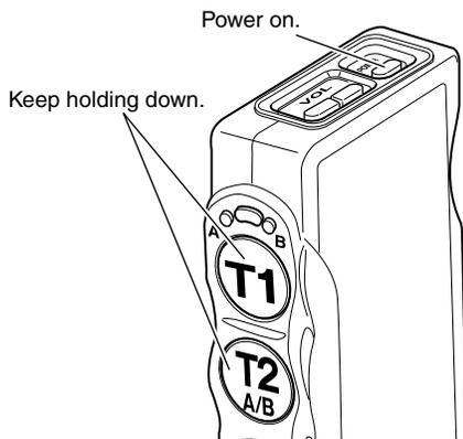
3. Press the T1 button, the Order Taker searches for the center module. You can hear "Connecting center module A" and the lane Indicator will blink yellow.
