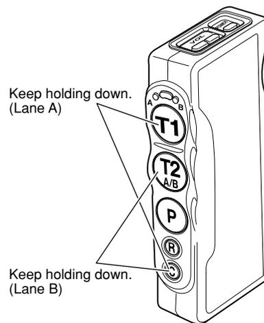
3. Press the P button while the power indicator keeps blinking in yellow. The ID that is registered for LANE A (or LANE B) is deleted.
