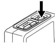
2. To delete an ID that is registered for LANE A, keep pressing the T1 and C buttons simultaneously and start up the power of Order Taker.
