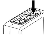
2. When LANE A is set in the manager mode, keep pressing the R and T1 buttons simultaneously and start up the power of Order Taker.
